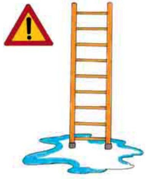
Fig. 24 - Do not lean the ladder on a slippery surface
