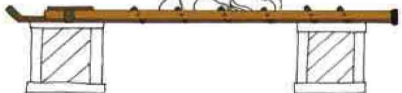
Fig. 9- Do not use the ladder as a platform or a gangplank
