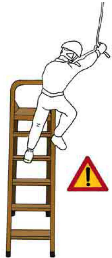
Fig. 10a - Positioning both feet on the ladder, taking care not to lose his balance
