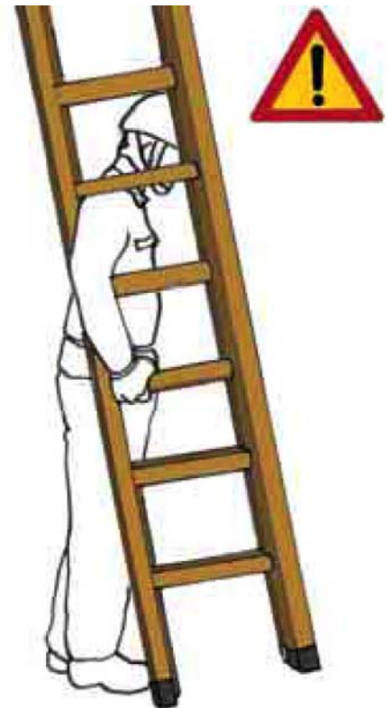
Fig. 6 - Incorrect method of carrying a ladder on one's own shoulder
