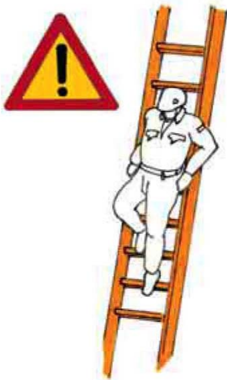
Fig. 40 - Incorrect ascent/descent procedure
