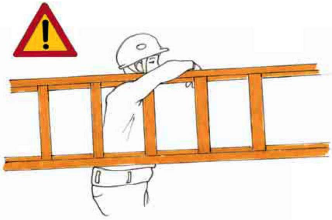
Fig. 22 - Wrong method to carry the ladder on one's own shoulder
