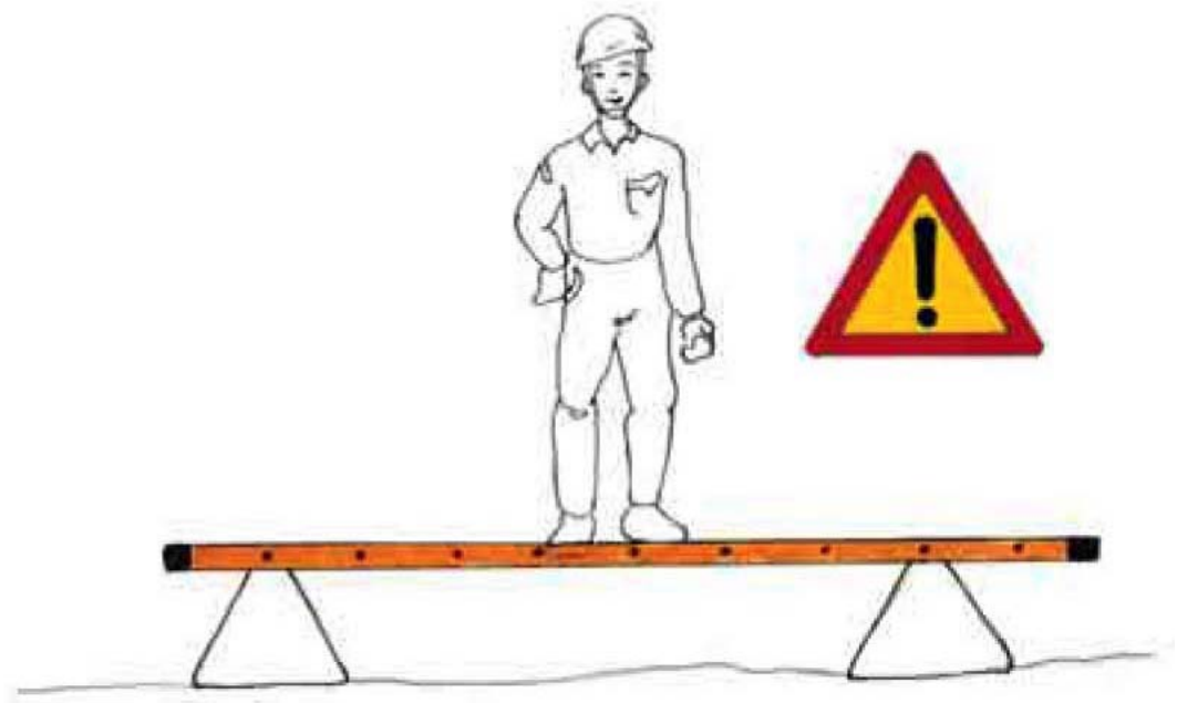
Fig 28 - Do not use the ladder as a scaffold or a gangplank
