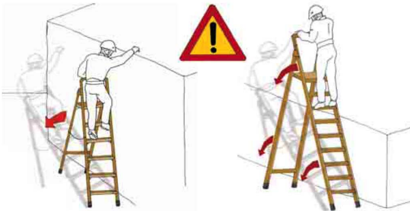
Fig. 4 - Misuse of the ladder: lateral position and system of access to a different place
