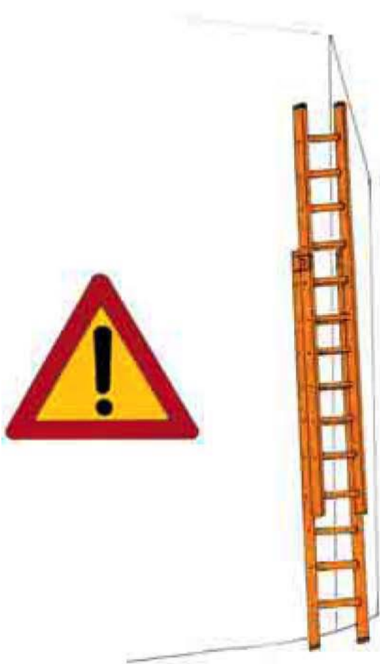
Fig. 18 - Wrong positioning of the ladder on a corner support
