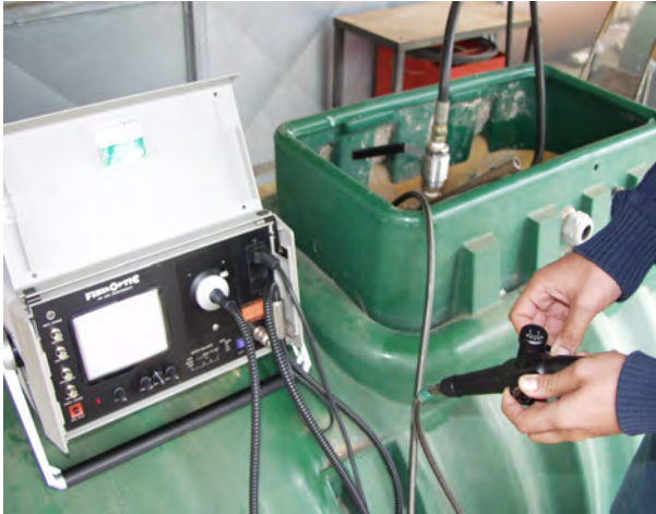
a) EV remoto intercapedine serbatoio GPL
